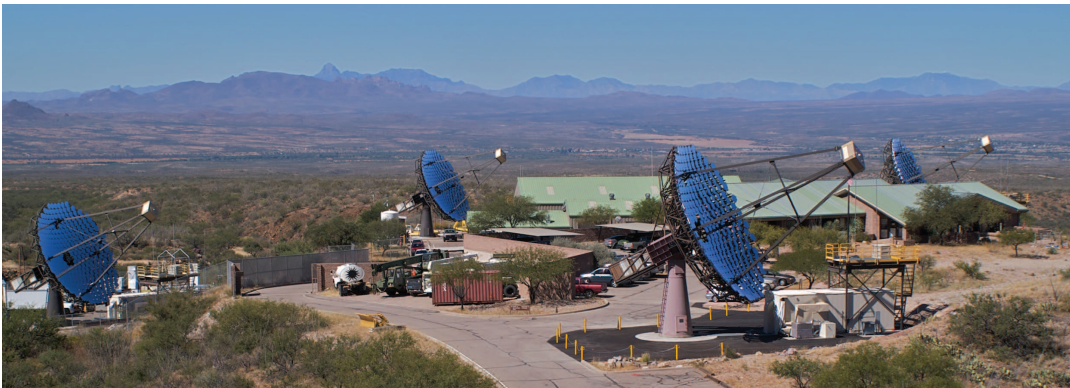
Fig. 6.6. Photograph of the four VERITAS 12-m diameter Cherenkov telescopes at the Mount Hopkins base camp in Arizona.
